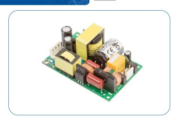
The ECP130 series is designed to minimize the no load power consumption and maximize efficiency to facilitate equipment design to meet the latest environmental legislation. Approved for medical and ITE applications, this range of single output AC-DC power supplies are packaged in a low profile 1.1" height with a foot print of just 2" by 3". The ECP130 provides up to 130 W force-cooled or | 100 W convection-cooled leading to very high power densities of 19.7 W/in³ or 15.1 W/in³ respectively.
