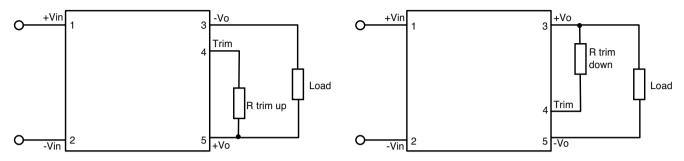
In order to trim the voltage up or down, connect the trim resistor either between the trim pin and -Vo for trim-up and between trim pin and +Vo for trim-down. The output voltage trim range is  $\pm 10\%$ . This is shown to the right.
