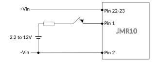
Module "On" if pin 1 is open circuit Module "Off" if pin 1 is connected to current source of 2-4mA, or a voltage of 2.2 to 12V is applied to pin 1 WRT pin 2.
