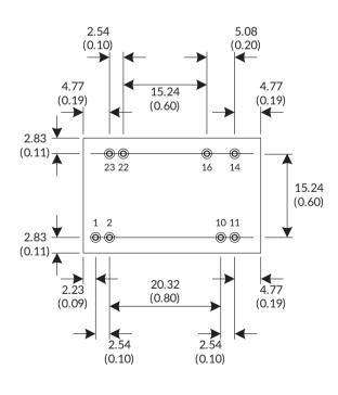
There should be at least 8mm distance between primary and secondary circuit.
